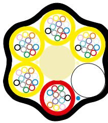
**Application:** Fiber optic cable designed to be used in cable ducts for backbone network installation in places not threatened by mechanical damage or rodent attacks. Suitable to be used in cable pipes.
