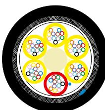
**Application:** Fiber optic cables intended for internal and external application in places without a threat of mechanical damage, however appropriate for places where there is a risk of rodent attacks. Cable suitable for installation within the wind farms and public areas with higher risk of fire.
